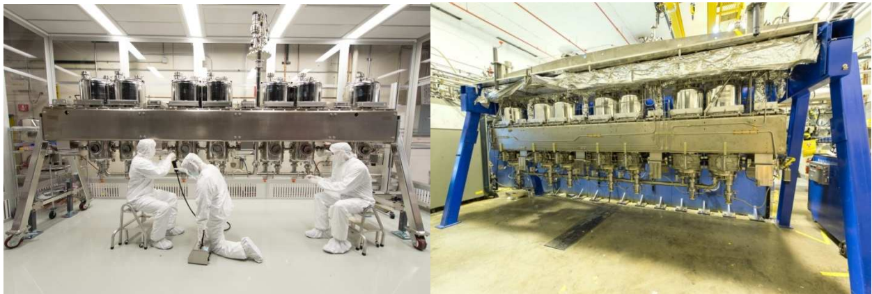
Figure 1: Left: seven 72 MHz SC cavities after final clean room assembly. Right: completed cryomodule string with cavities, couplers, tuners, alignment and cryogenics systems.
